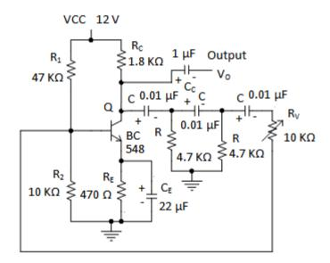
From the given component values, the frequency of oscillation
