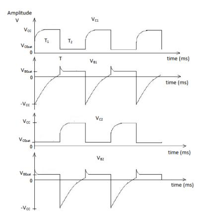
ON time of Q1, T1 = OFF time of Q1, T2 = Time period, T = T1 + T2 = Frequency,  $f = \frac{1}{T}$  =
