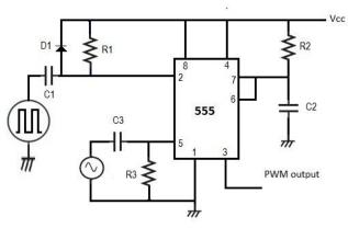
$R_1$ =1.2K,  $R_2$ =4.7K,  $R_3$ =10K,  $C_1$ = 0.001 $\mu$ F,  $C_2$ =0.1 $\mu$ F,  $C_3$ =10 $\mu$ F
