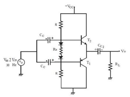
R=1K $\Omega$ , R<sub>B</sub>=1K $\Omega$ , R<sub>L</sub>=1K $\Omega$ , C<sub>C1</sub>=220µF, C<sub>C2</sub>=100µF, D<sub>1</sub>&D<sub>2</sub>=1N4001, T<sub>1</sub>=SK100, T<sub>2</sub>=SL100 & Vcc-10V
