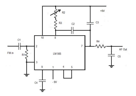
$C_1=0.1\mu F$ ,  $R_1=620\Omega$ ,  $R_2=10K$ ,  $R_3=4.7K$ ,  $C_2=.001\mu F$ ,  $R_4=1K$ ,  $C_3=.1\mu F C_4=0.001\mu F$
