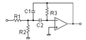
IC= 741, R1 =  $4.7k\Omega$ , R2 =  $4.7k\Omega$ , R3 =  $5.6k\Omega$ , C1 = 0.0047uF, C2 = 0.01uF
