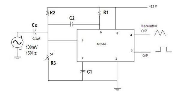
$R_1$ =6.8K,  $R_2$ =10K,  $R_3$ =47K,  $C_c$ =0.1 $\mu$ F,  $C_1$ =0.01 $\mu$ F,  $C_2$ =0.001 $\mu$ F
