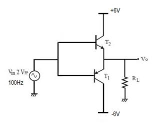
$T_1 = SK100, T_2 = SL100, R_L = 1K\Omega$
