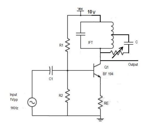
R<sub>1</sub>=82K, R<sub>2</sub>=18K, R<sub>e</sub>=1K, Pot=47K, C<sub>1</sub>=0.1µF, C=330pf
