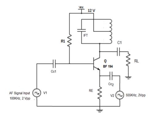
R1=680K, R<sub>E</sub>=1.2K, C<sub>C1</sub>=0.1 $\mu$ F, C<sub>C2</sub>= 0.1 $\mu$ F, C1=10 $\mu$ F, RL= 1K
