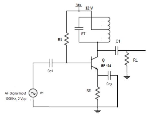
R1=680K,  $R_E$ =1.2K,  $C_{C1}$ =0.1µF,  $C_{C2}$ = 0.1µF, C1=10µF, RL= 1K
