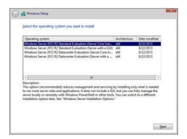
This screen enables you to select either the complete installation of Windows Server 2012 R2 or the Server Core option.
