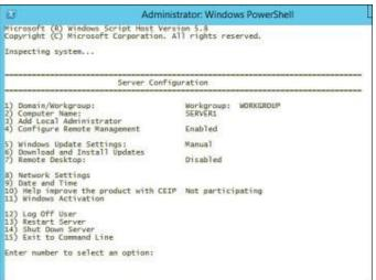
The Sconfig.cmd utility enables you to perform many basic configuration actions on a Server Core computer.
